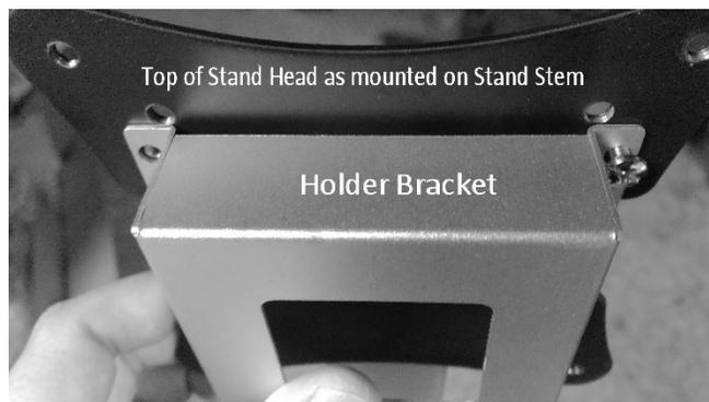
4. Install on the Stand Head onto the Stand Pole by using supplied Allen Wrench, removing bolt, nut, and spacers. Align the spacers as shown in Stand Pole. Then insert and tighten bolt and nut, ensuring nut is captured by nut profile in Stand Head. Tighten enough so that the Stand Head is stiff to move on joint but not immovable:
