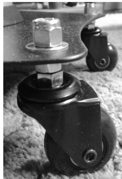
2. Install Casters to Stand Base as shown with washer on top covering the countersunk depression, using supplied wrench to tighten (5 casters):
