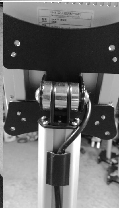
The battery cable is mounted like this to allow a plastic bag to be placed over the battery and secured by the Velcro straps for weather resistance.
