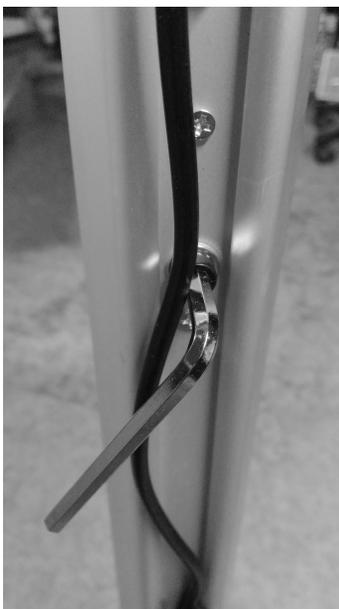
8. Raise Stand Pole section by using the supplied Allen wrench to loosen the (2) rear setscrews, and then lift smaller pole portion to as high as it will go, then retighten the setscrews:
